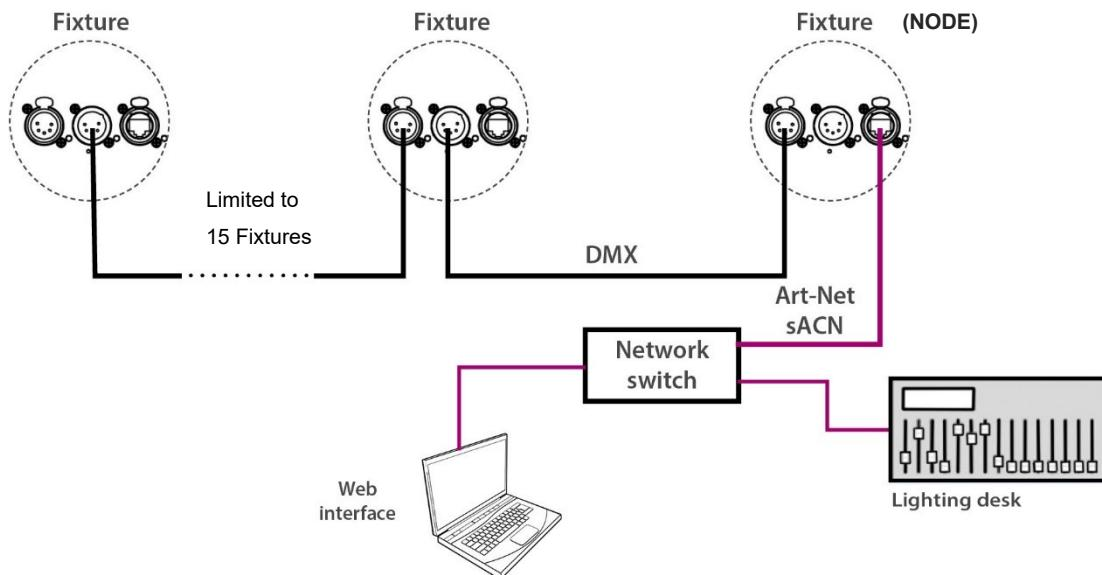
A node has now been implemented. This function converts an ethernet protocol, in our case sACN and Art-Net 3/4 into a DMX signal but with the particularity to carry RDM functionalities as well.
