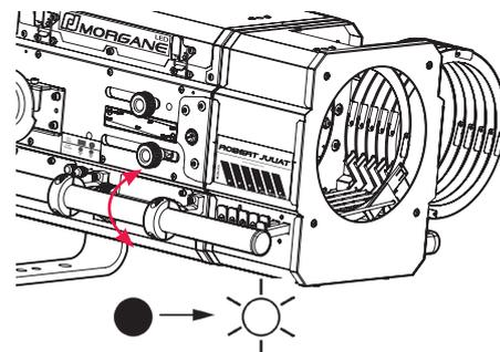
Step 4 - The light beam zoom and focus can be set by using the control knobs A & B /
