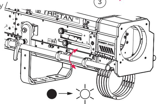
Step 4 - The light beam zoom and focus can be set by using the control knobs A & B /
