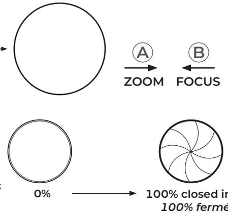
Step 5 - The beam size can be adjusted by using the iris handle /
